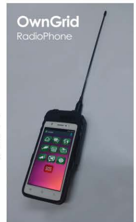
Fig.3 OwnGrid enables seamless connectivity over sea. It helps fishermen find the best locations for fishing. OwnGrid provides multiple applications, such as navigation, weather prediction, fishing areas, as well as online chatting. The product is also able to report any SOS condition.
