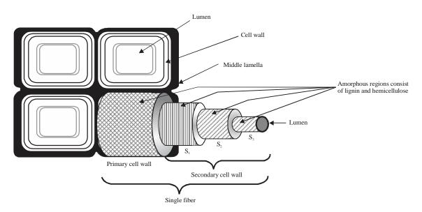
Fig. 1: Sceme of the basic three structure of natural fiber of the plant raw materials
