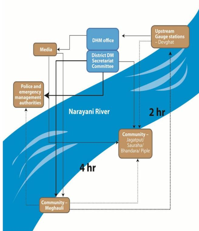
**Figure 1 : Mechanisms of the early warning system**
