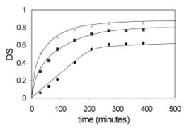
**Fig. 4.** DS as a function of the reaction time for different temperatures.  $55^{\circ}$ C ( $\blacktriangle$ ),  $45^{\circ}$ C ( $\blacksquare$ ),  $35^{\circ}$ C ( $\blacklozenge$ ).
