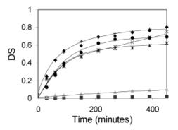
**Fig. 1.** DS of cassava starch for different solvents as a function of the reaction time. Organic liquids: methanol ( $\blacksquare$ ), ethanol ( $\blacktriangle$ ), 1-butanol (x), 2-butanol (\*), 1-propanol ( $\bigcirc$ ), *tert*-butanol (+), isopropanol ( $\diamondsuit$ ).
