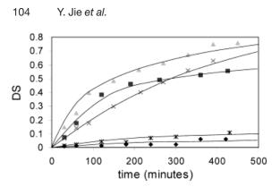
**Fig. 3.** DS as a function of the reaction time for different water intakes. 4% H<sub>2</sub>O ( $\blacklozenge$ ), 7% H<sub>2</sub>O ( $\blacksquare$ ), 10% H<sub>2</sub>O ( $\blacktriangle$ ), 13% H<sub>2</sub>O (x), 16% H<sub>2</sub>O (\*).
