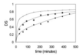
**Fig. 6.** DS at different  $n_{\text{NaOH}}/n_{\text{SMCA}}$  ratios as a function of the reaction time.  $n_{\text{NaOH}}/n_{\text{SMCA}}$ : 0.75 ( $\blacklozenge$ ), 1.0 ( $\blacksquare$ ), 1.50 ( $\blacktriangle$ ).
