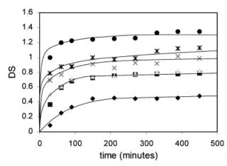
**Fig. 7.** DS at different DS<sub>t</sub> levels as function of the reaction time. DS<sub>t</sub>: 0.8 ( $\blacklozenge$ ), 1.1 ( $\blacksquare$ ), 1.2 ( $\blacktriangle$ ), 1.4 (x), 1.6 (\*), 2.5 ( $\bigcirc$ ).
