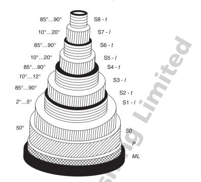
16.3 Polylamellate structure of a thick-walled bamboo fibre (ML = middle lamella, P = primary wall, S = secondary wall) (Liese, 1985).
