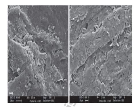
*16.4* SEM micrographs of bamboo fibre–polypropylene interface: (a) without maleic anhydride grafted polypropylene (MA-*g*-PP) and (b) with MA-*g*-PP for 50 vol% of bamboo fibre (Chattopadhyay *et al.*, 2011a, © 2010 Wiley Periodicals, Inc.).
