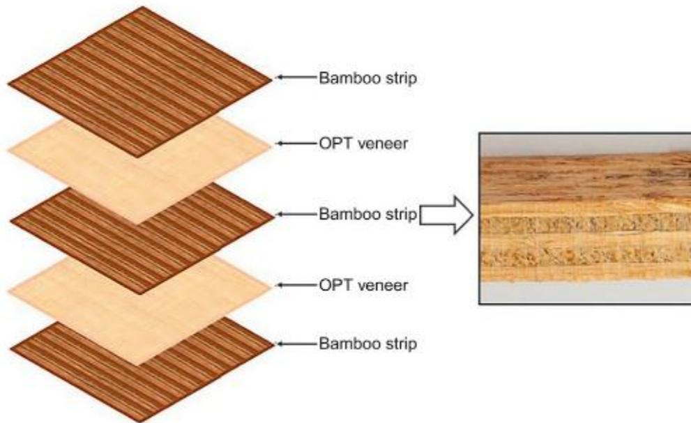
**Fig. 14.5** Laminated bamboo strips hybrid with OPT veneer biocomposites (LBHC).
