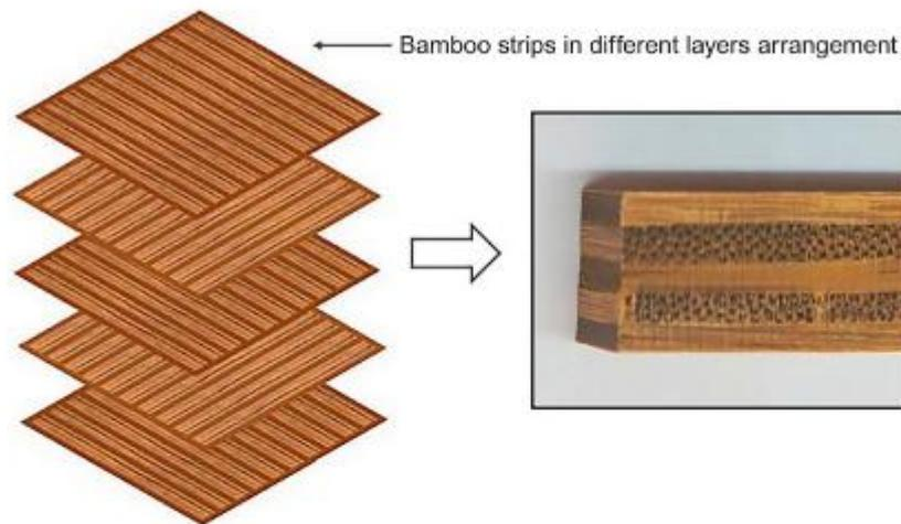
**Fig. 14.4** Laminated bamboo strips bio-composites in different layers arrangement.
