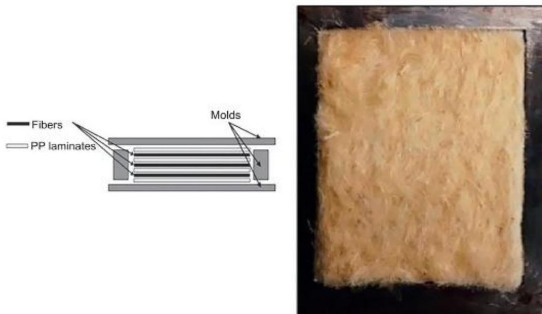
**Fig. 14.6** Pineapple leaf fibers reinforced polymer composites [67].
