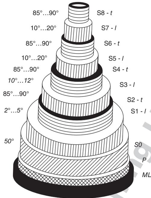
16.3 Polylamellate structure of a thick-walled bamboo fibre (ML = middle lamella, P = primary wall, S = secondary wall) (Liese, 1985).
