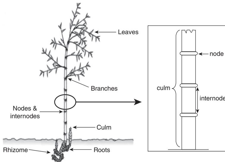
16.1 Structure of a bamboo (Sakaray *et al.*, 2012).
