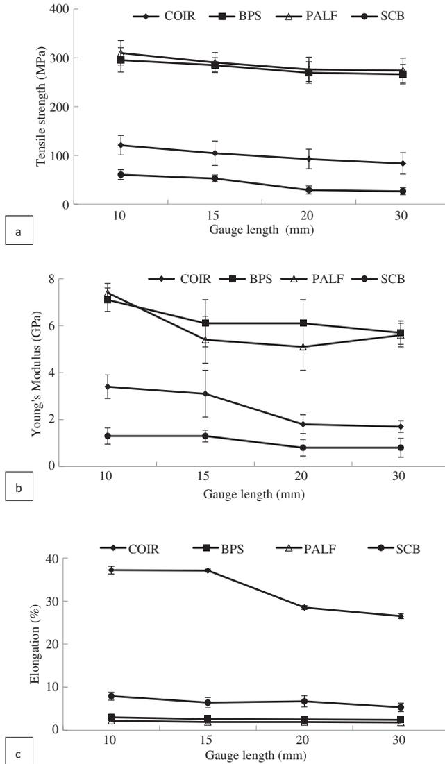
FIGURE 6 Tensile properties, i.e., (a) tensile strength, (b) Young's modulus, and (c) elongation, as a function of gauge length for COIR, BPS, PALF, and SCB fiber.
