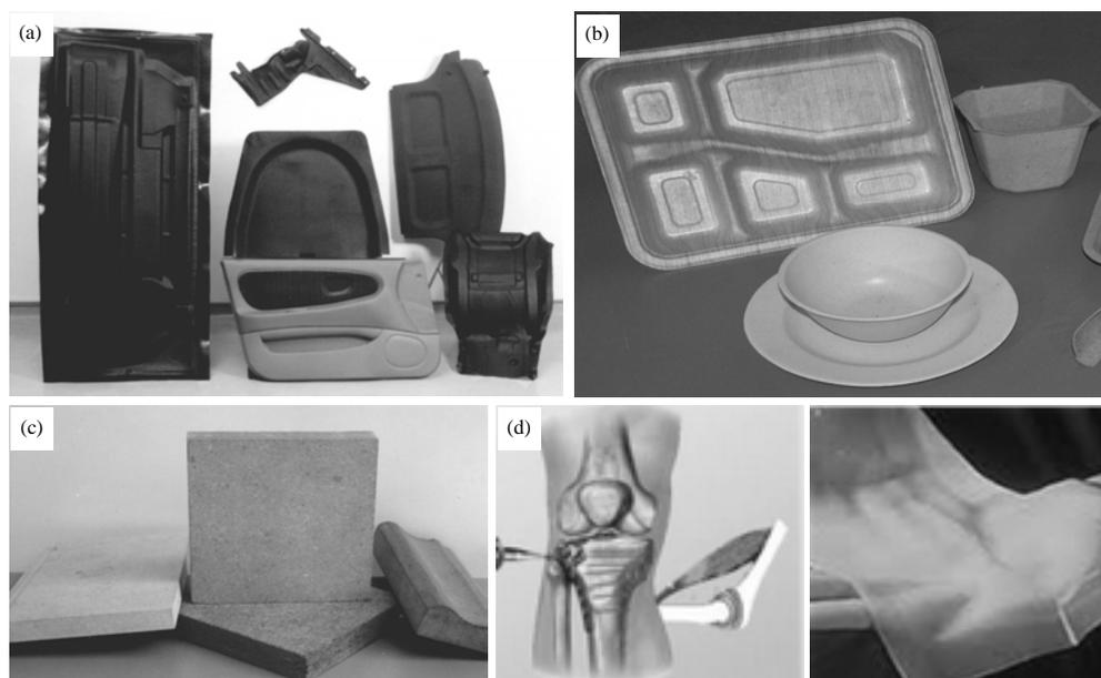
Fig. 3(a-d): Various applications of agro-based biocomposite, (a) Automotive component, (b) Food packaging, (c) Building component and (d) Medical applications, sources: Dungani *et al.* (2014) and Lina *et al.* (2011) with permission
