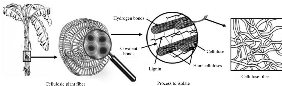
Fig. 2: Schematic principle of isolation process isolate from cellulosic plant fiber to cellulose fiber
