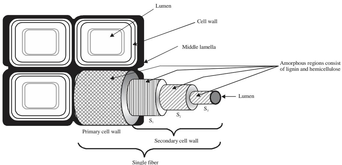
Fig. 1: Scheme of the basic three structure of natural fiber of the plant raw materials
