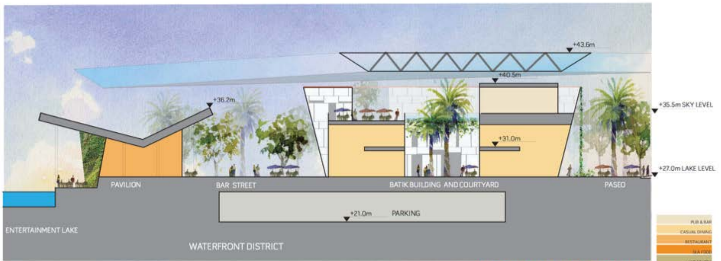
SECTION THROUGH BAR STREET AND PASEO
