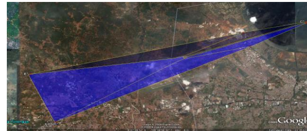
OAS (Obstacle Assessment Surface) Template for Runway 25R Aircraft Category C/D
