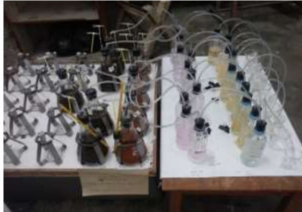
Figure 2 Experimental set-up under anaerobic condition
