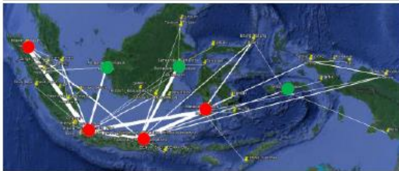
Optimized network based on port performance aspirations and cost-minimization has transshipments and features sub-hubs
