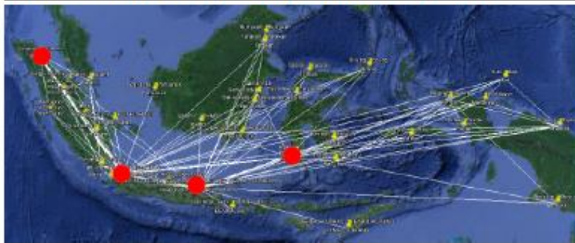
Optimized network based on port performance aspirations and cost-minimization has transshipments and features sub-hubs
