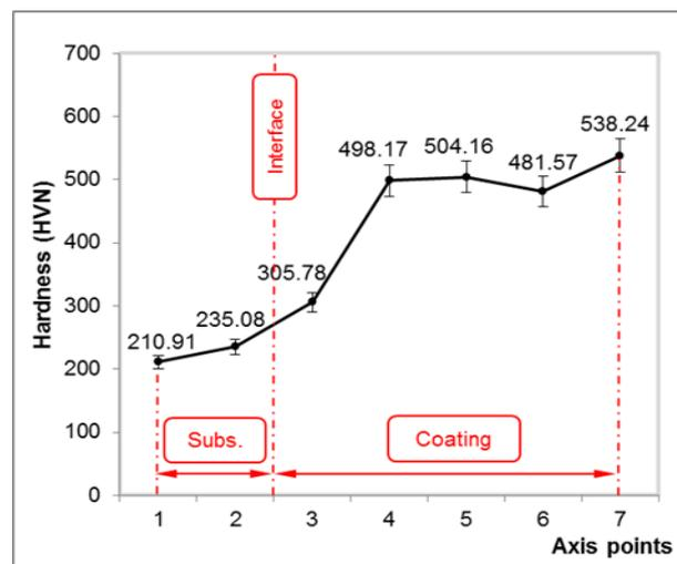
**Figure 9.** Microhardness profile of MMC 2 components coating.
