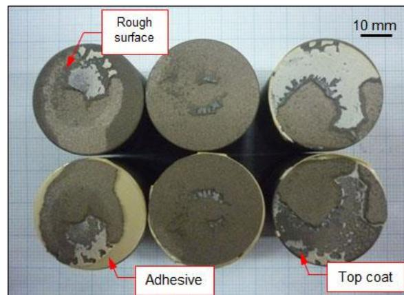
**Figure 11.** Coating fracture mode of MMC 2 components is cohesive failure, top coat delamination from its bond coat.
