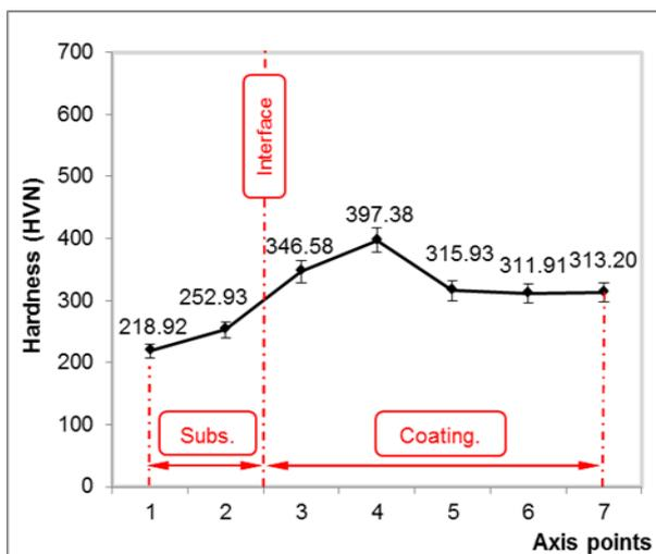
**Figure 8.** Microhardness profile of MMC 3 components coating.
