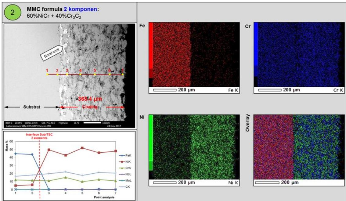
**Figure 5.** SEM micrograph of HVOF spray MMC 2 components, constituent element mapping, and point analysis.
