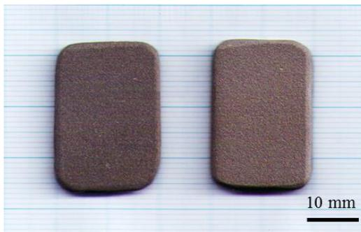
**Figure 3.** The as-coated result of MMC 3 components and 2 components using TECKNOTHERM HVOF 2007 thermal spray machine and spray gun Hipojet-2700.
