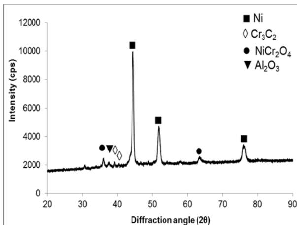
**Figure 6.** X-ray diffraction pattern of MMC 3 components coating.
