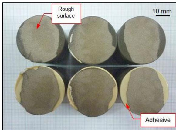
**Figure 10.** Coating fracture mode of MMC 3 components is adhesive failure, bond coat were detached more than 80% from substrate.
