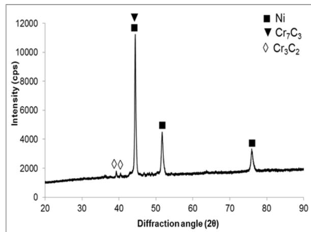
**Figure 7.** X-ray diffraction pattern of MMC 2 components coating.
