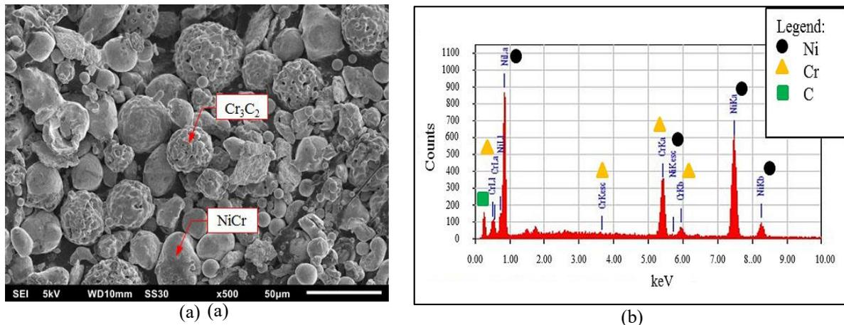
**Figure 2.** SEM micrographs of NiCr matrix composites powder with Cr<sub>3</sub>C<sub>2</sub> reinforcement; (a) feedstock; (b) EDS spectra of MMC 2 components feedstock.
