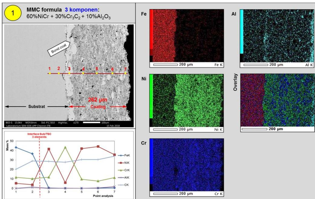
**Figure 4.** SEM micrograph of HVOF spray MMC 3 components, constituent element mapping, and point analysis.
