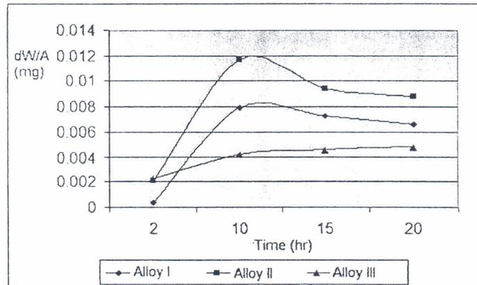
Figure 20. Weight change ( gr/cm2) with times of alloys I, II and III oxidized at 900°C for 25 hours.
