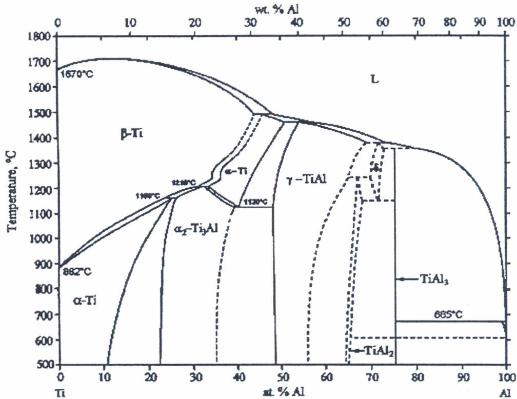
Figure 1. Phase diagram of binary Ti – Al alloys<sup>[3]</sup>
