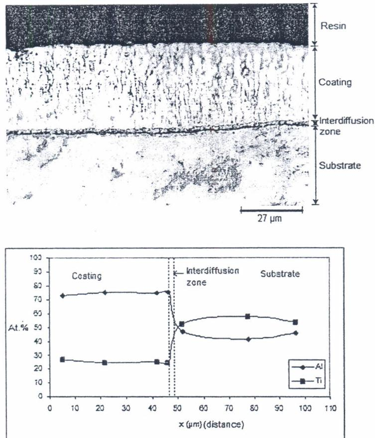
Figure 7. Microstructure and concentration profiles of Ti and Al of as coated binary  $\alpha_2\text{-Ti}_3\text{Al}/\gamma\text{-TiAl}$  alloy.
