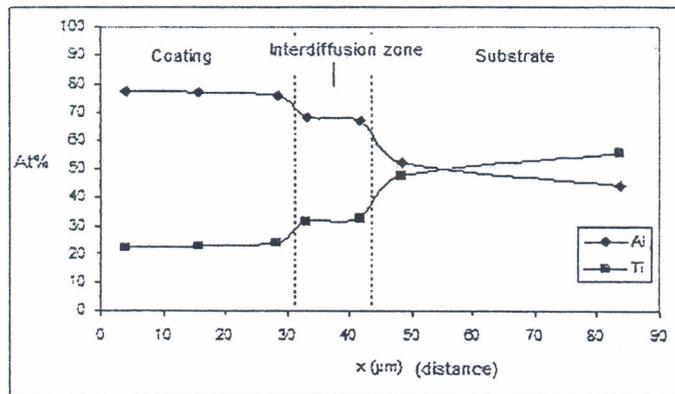
Figure 9. Microstructure and concentration profiles of Ti and Al of coated binary  $\alpha_2$ -Ti<sub>3</sub>Al/ $\gamma$ -TiAl alloy heated at 900°C for 10 hours.
