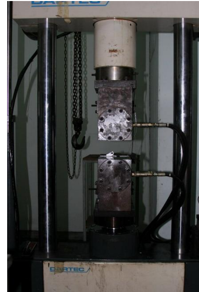
Fig. 1. Configuration of CT-Spesimen and Universal Testing Machine used in this study.
