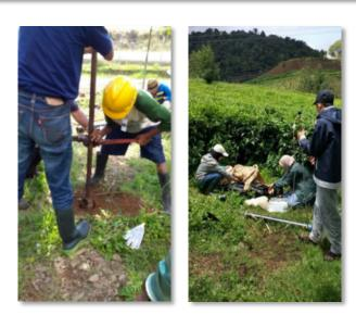
Drilling activity to make monitoring point for Radon and Mercury also for gas sampling, total there are 18 holes were dedicated for monitoring points (left).
