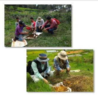
Soil sampling and soil mineralogy description at site. Soil samples were brought and analyzed using BAGUS instrument at ITB. Mineralogy and soil geochemistry are very useful to determine alteration type and inferred temperature.
