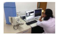
Scanning Electron Microscope (SEM) observation by researcher, the SEM including X-ray energy Dispersive Spectrometry system use for observing mineral and structure of the mineral, including element map of the samples.
